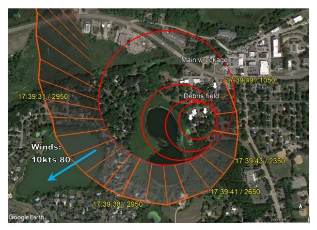
**Figure 4.** Final turn with time and altitudes (in msl). The red circles near the center of the figure depict the radius of the airplane's final left turn at four different points.
